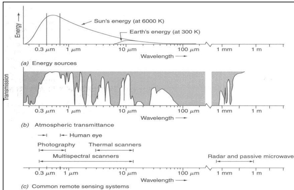
Figure 7: Spectral characteristics of (a) energy sources, (b) atmospheric transmittance, and (c) common remote sensing systems
