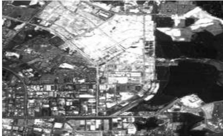
Fig. 7 Panchromatic image extracted from SPOT PAN sensor with ground resolution 10 m. (Source:[http://www.crisp.nus.edu.sg/~research/tutorial/opt\\_int.htm](http://www.crisp.nus.edu.sg/~research/tutorial/opt_int.htm)).
