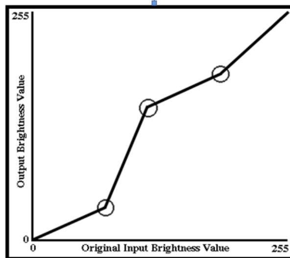
Fig(7): Logic of a piecewise linear contrast stretch:Source: <http://www.r-s-c-c.org/node/244>
