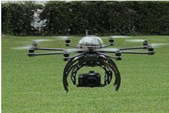
Figure 4: A drone carrying a camera for aerial photography (<http://www.en.wikipedia.org>).
