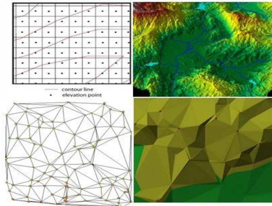
Fig 1. Illustration of DEM and TIN
