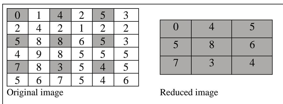
Fig (11): Logic of a simple 2x integer reduction. Source: Self
