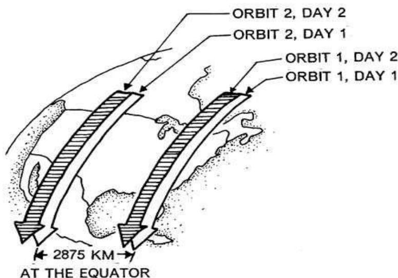
Fig. 18 Orbital shift of a typical sun- synchronous satellite
