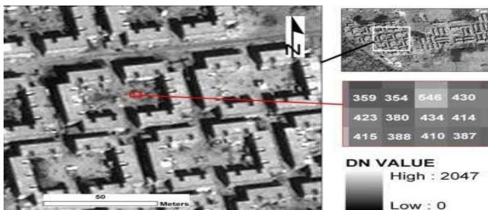
Fig. 19 An example of an 11 bit image. Each pixel contains a value between 0 and 2047 according to the strength of the EMR measured at the sensor; values termed as Digital Numbers (DN); (Lillesand Kiefer, 1987).
