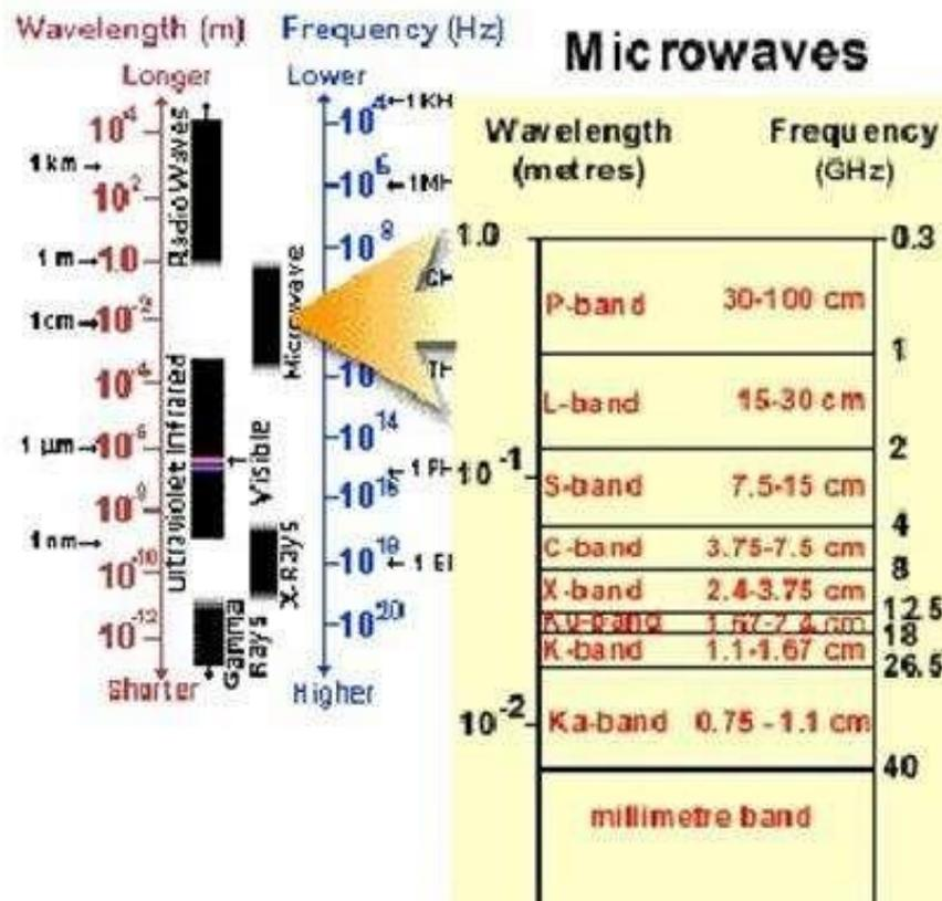
Fig. 15 The microwave region of the electromagnetic spectrum; source: Fundamentals of Remote Sensing by CCRS, Canada.
