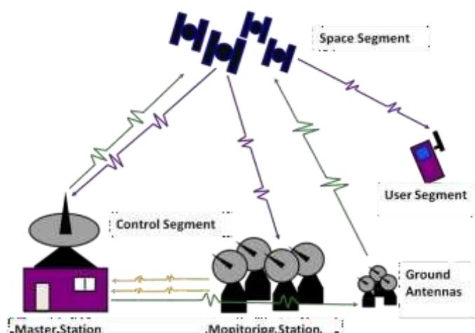
Fig. 9: Three segments of the GPS (Source: Texas Tech University Departments)
