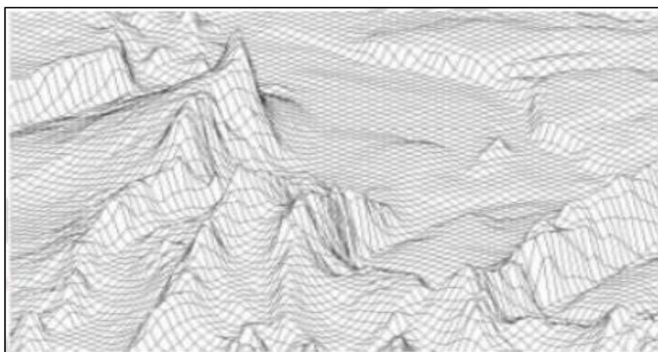
**Figure 3: A Digital Elevation Model showing continuous coverage of slope, aspect, and elevation in a raster grid across an entire area. This area is the east side of the Cascade Mountains in west-central Washington State. Each regular grid cell is 1 km on a side. Figure developed and provided by Steve Brown at the University of Montana**
