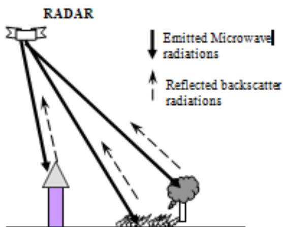
Fig. 12. Active microwave sensor.
