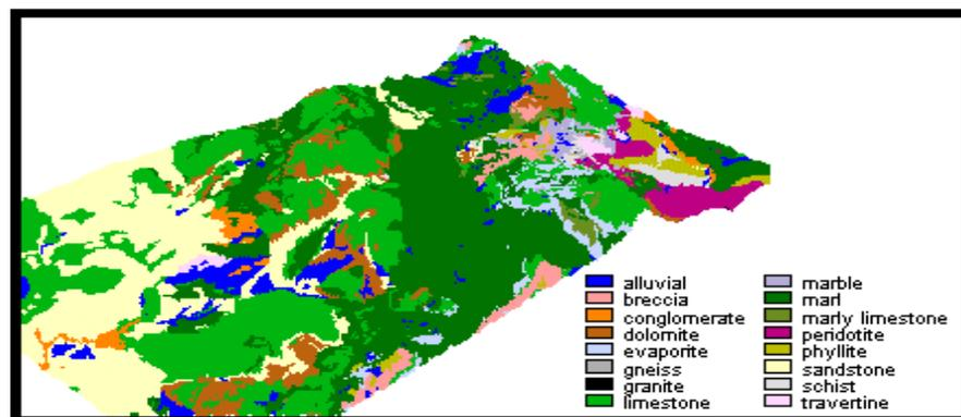
Fig 15: Lithological map draped over the topography
