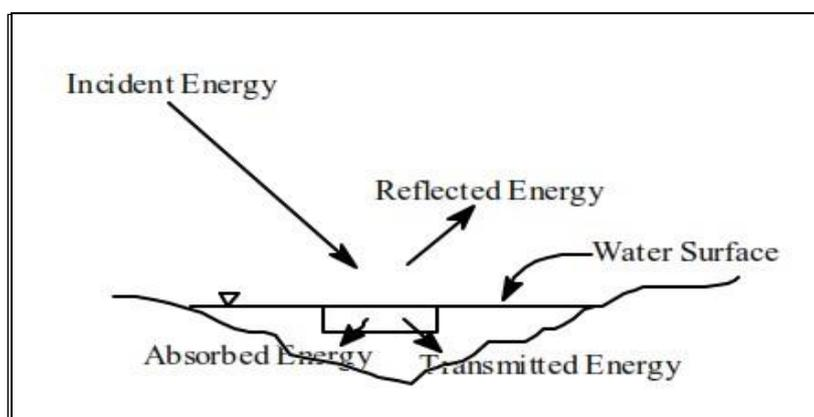
Figure 8: Basic interactions between electromagnetic energy and an Earth surface feature
