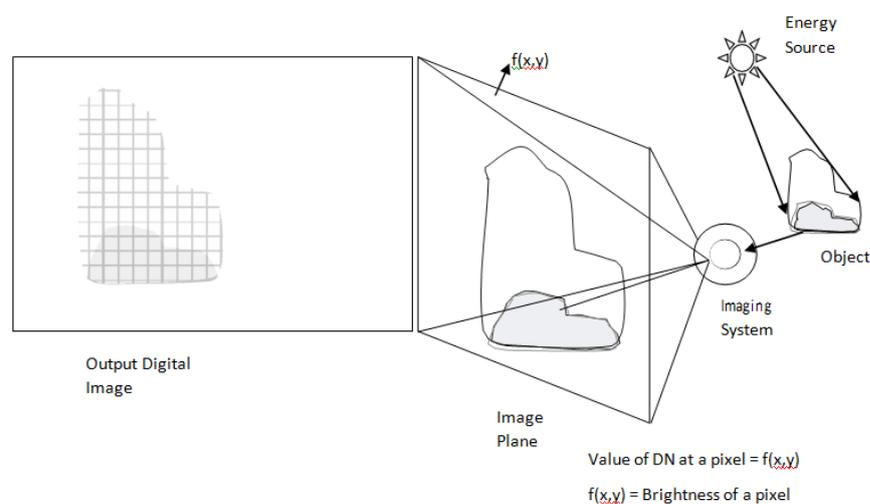
**Figure 1.** Representation of a 2-D digital image
