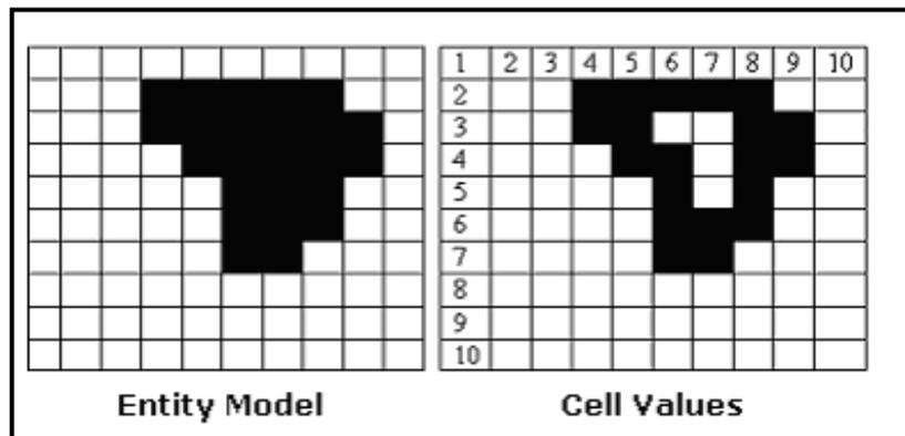
Figure 1: Locating Grid Cells for Chain Coding in Raster GIS
