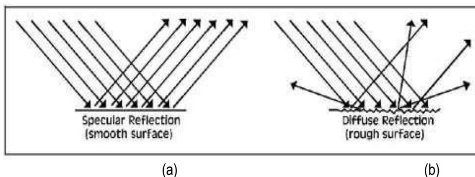
Fig. 17 (a) Specular reflection over a smooth surface and (b) diffuse reflection over surface irregularities.
