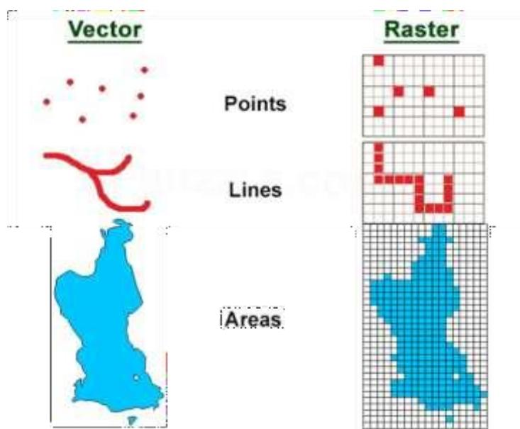
Fig. 2: Representation of data in GIS (Vector and Raster format)
