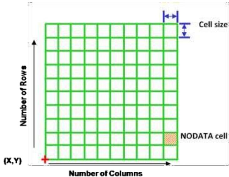
Fig. 3: Definition of a Grid in GIS
