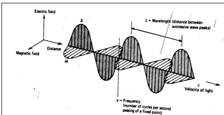
Figure 3: Electromagnetic wave. Components include a sinusoidal electric wave (E) and a magnetic wave (M) perpendicular to each other as well as to the direction of propagation.
