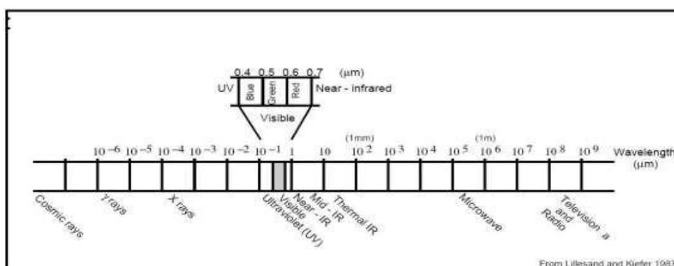
Fig. 10 The electromagnetic spectrum (Lillesand Kiefer, 1987).
