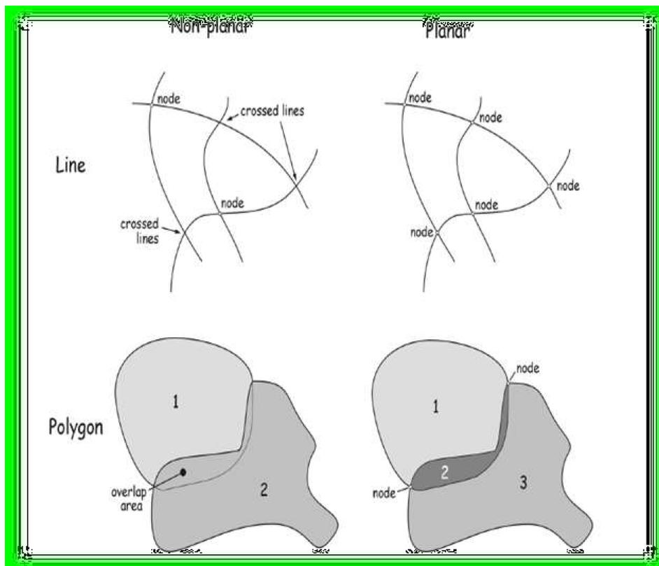
Figure 9: Non planar and Planar topology in Lines and polygons
