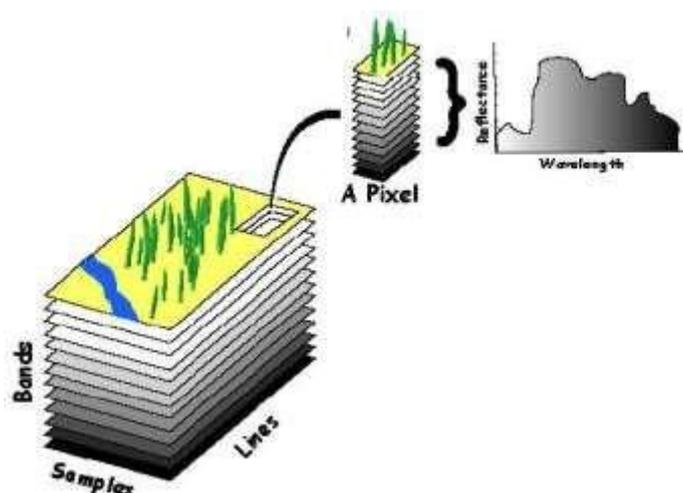
Fig. 10 Images acquired simultaneously in 200 or more spectral bands and the wavelength range depicted by the pixels; Source: Basics of remote sensing, Unit I; ESA website.
