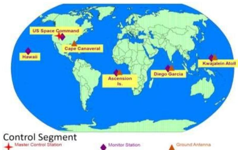
Fig. 11: Monitor Stations and Master Control Stations of GPS
