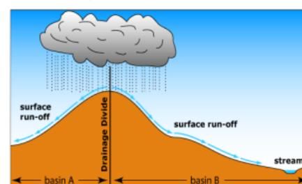
Figure 02: Drainage divides
