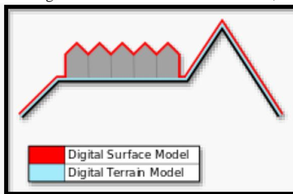
Fig 4: Surfaces represented by a Digital Surface Model include buildings and other objects. Digital Terrain Models represent the bare ground.
