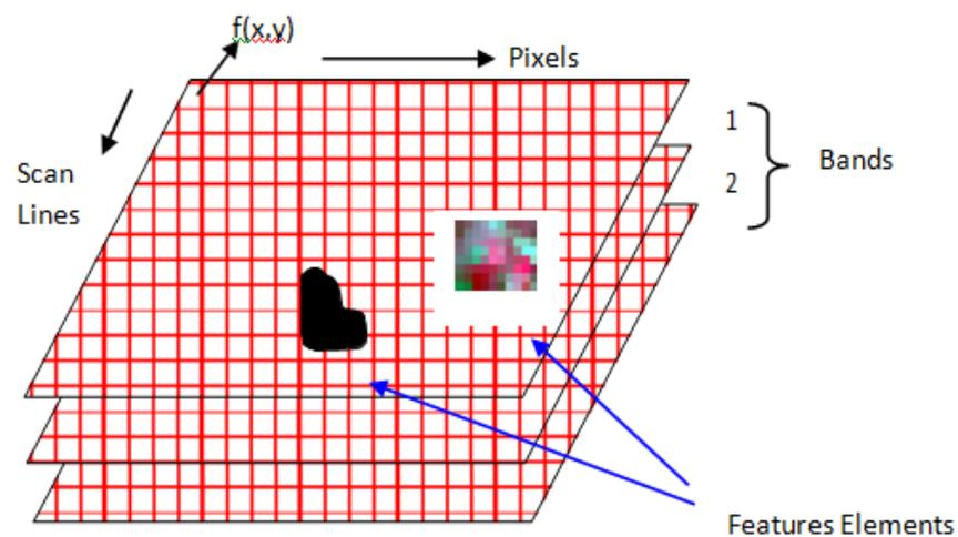
Figure 4. Structure of a Multispectral Image and feature elements
