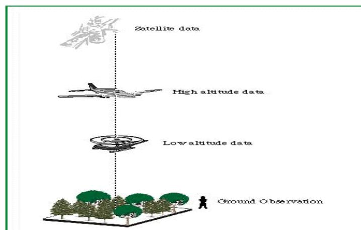
Figure 21. : Multistage remote sensing concept
