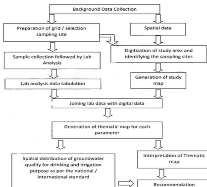
**Figure 3: Flow chart for application of remote sensing and GIS technique for water pollution study**
