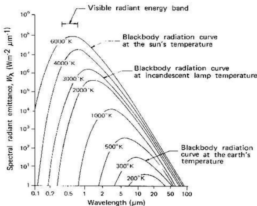
Fig. 16 Spectral curves showing relative intensities of radiation (radiances) as a function of wavelength different materials having varying temperature.
