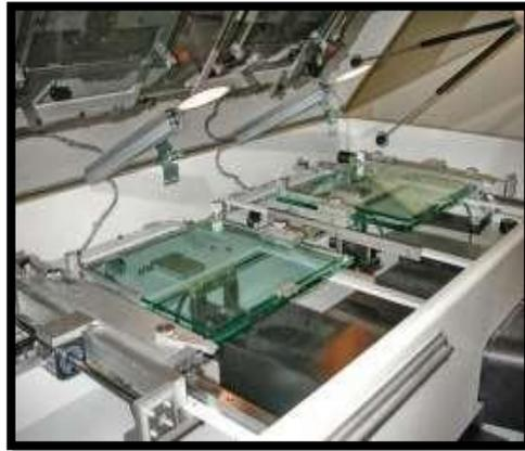
Fig B: Alpha 2000 stereoplottor
