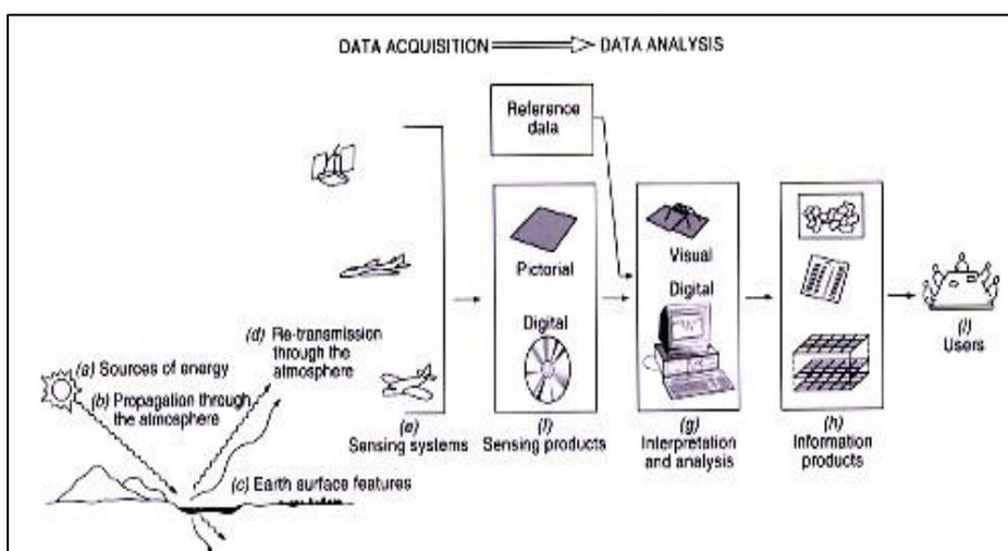
Figure 2: Electromagnetic remote sensing of Earth resources
