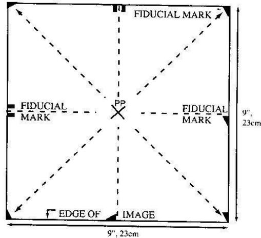
Figure 7: The image showing fiducial marks (<http://www.hosting.sonet.ca>)
