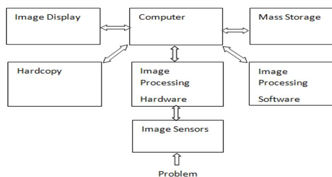
Figure 2. Essential components of a typical image processing system
