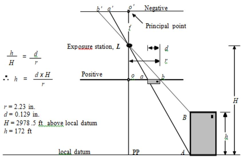
Fig 3: Measurement of height of the object from relief displacement
