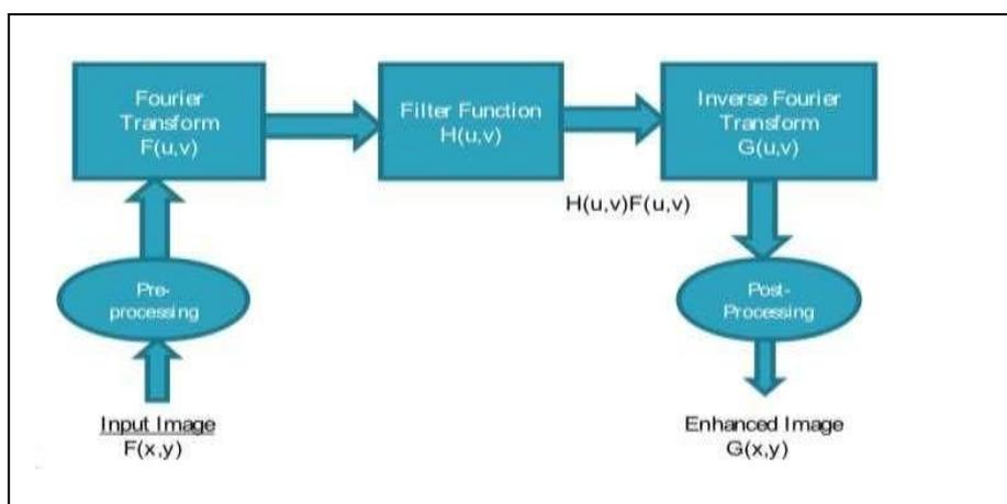
Fig (4): Filtering operation in frequency domain
