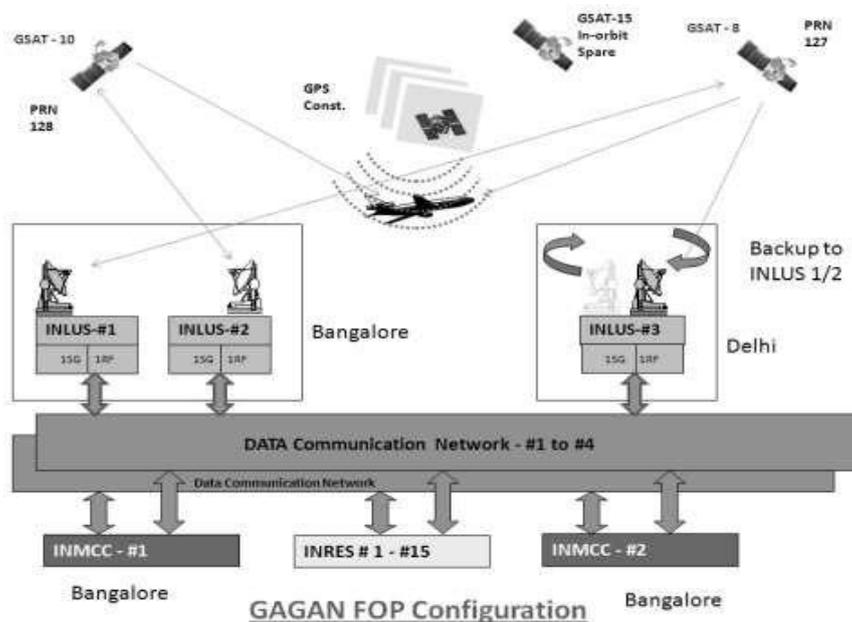
Fig. 13: GAGAN: System of operation
