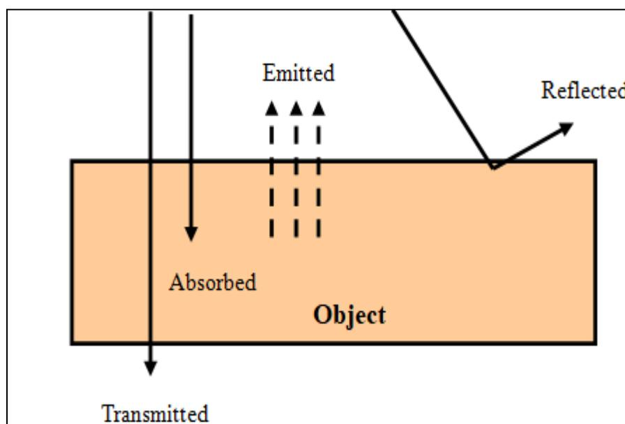
Fig. 16. Interaction of electromagnetic radiation with the surface or object.
