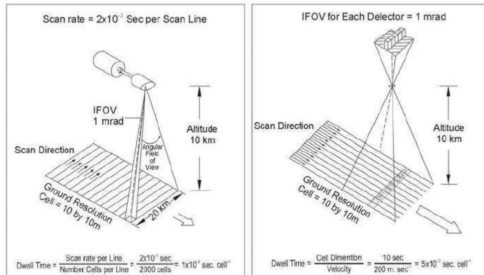
Fig. 9 (a) Whiskbroom scanner(b) Pushbroom scanner
