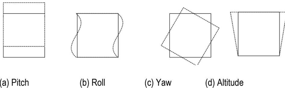
Figure 5. Effect of platform attitude errors
