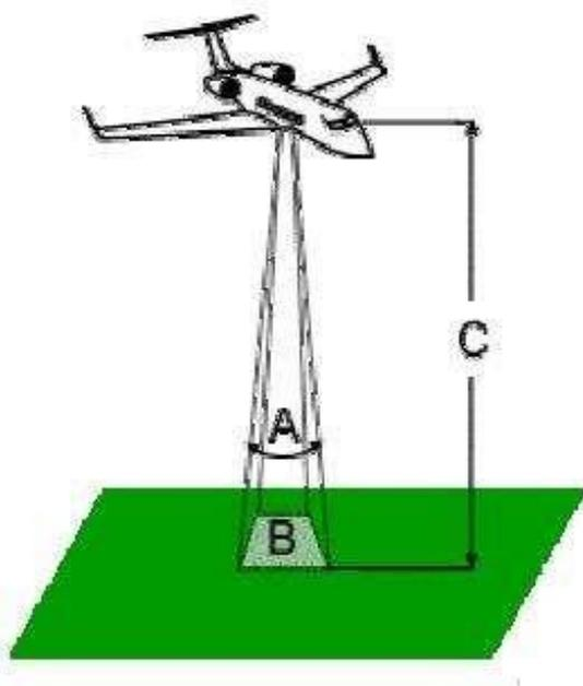
Fig. 8 Instantaneous Field of View (IFOV) for a typical scanner.
