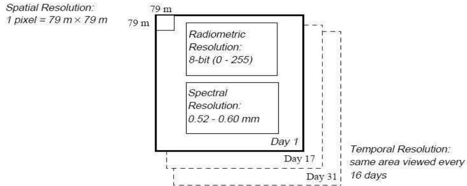
Fig. 20. Landsat TM—Band 2 (Four Types of Resolution); Source: EOSAT.
