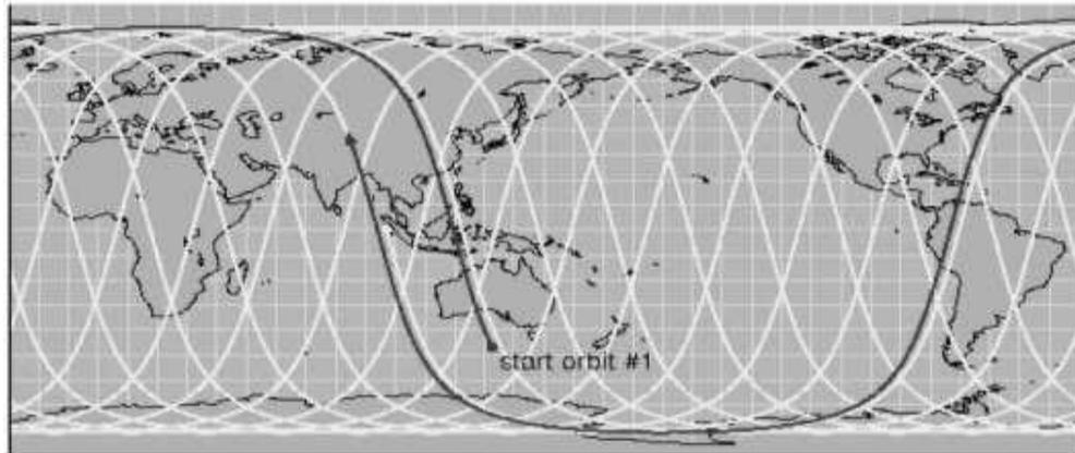
Fig. 19 Orbit of sun synchronous satellite.
