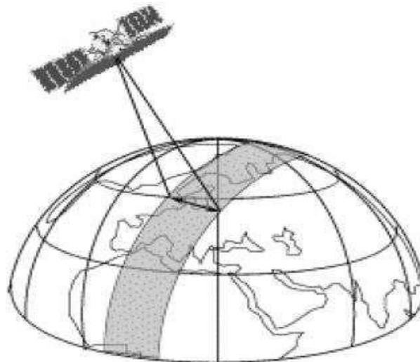
Fig. 20 Swath traced by polar orbiting satellite; source: Canada centre for remote sensing.
