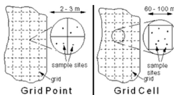
Fig. 14: Types of grid sampling
