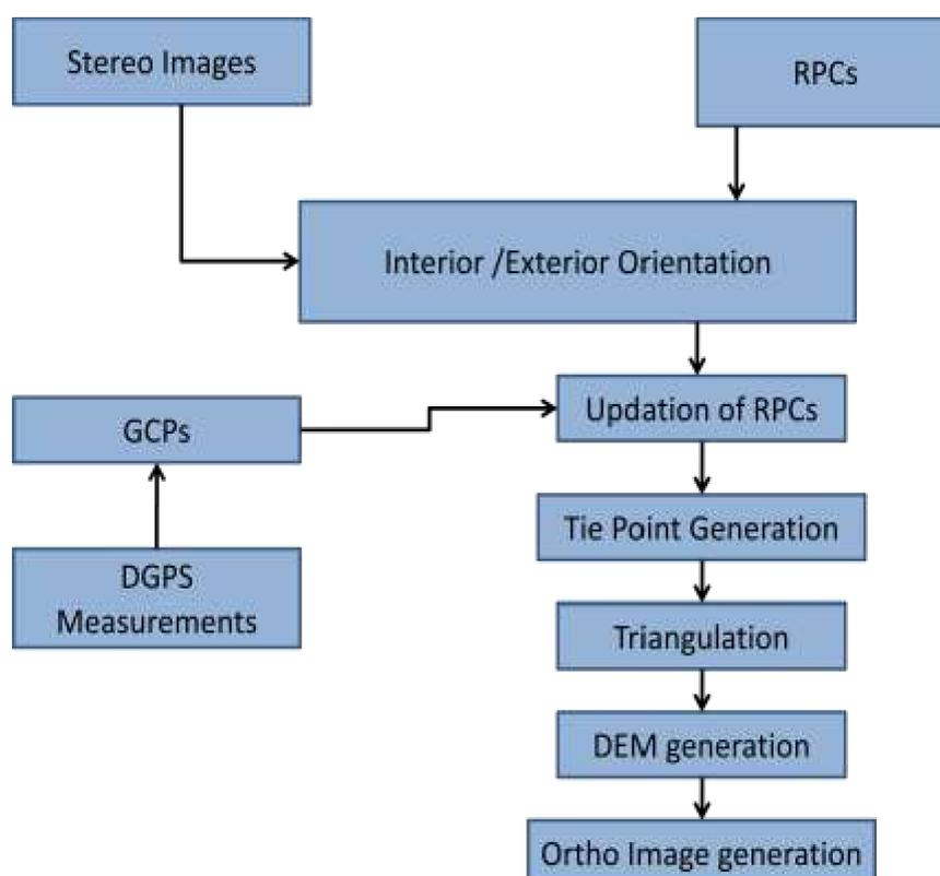
Fig 7: Flowchart for orthoimage generation
