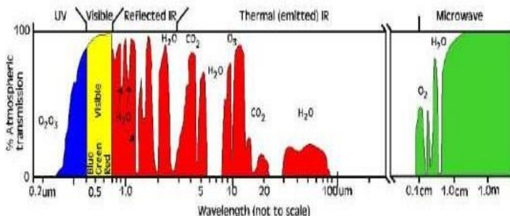
Fig. 14. Atmospheric windows with wavelength on x-axis and percent transmission measured in Hertz on y-axis. High transmission corresponds to an atmospheric window which allows radiations to penetrate electromagnetic radiation to penetrate the earth's atmosphere.
