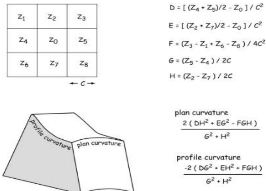
Fig 4. Estimation of Profile and plan curvature
