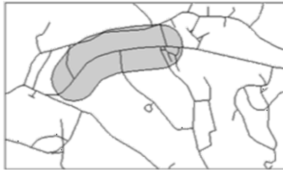
Figure 4.3 Buffering around a selected line feature
