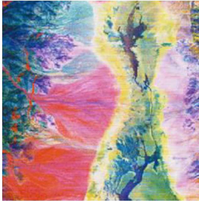
Figure 3.8: Thermal image of TAMS pertaining to Death Valley California. FCC of Band 1 –blue (8.2 - 8.6 \mu m), Band 3 -green (9.0 - 9.4 \mu m) and Band 5-red (10.2 - 11.2 \mu m)
