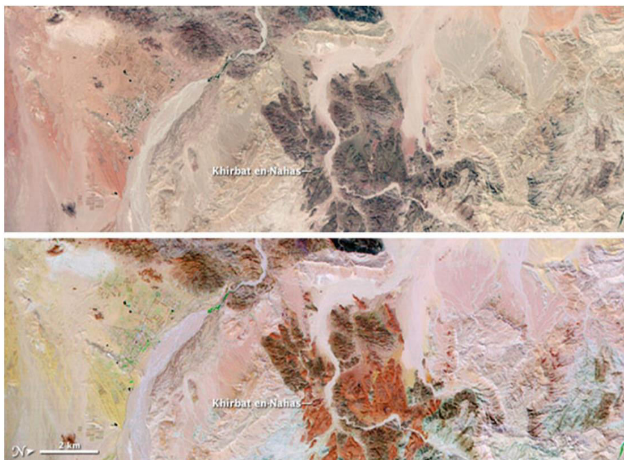
Fig. 4.7 Hyperion hyperspectral image over Khirbaten-Nahas, Jordan. This area host ancient copper mine, smelting sites and different rock types which was identified and mapped by hyperspectral data(NASA, 2016).
