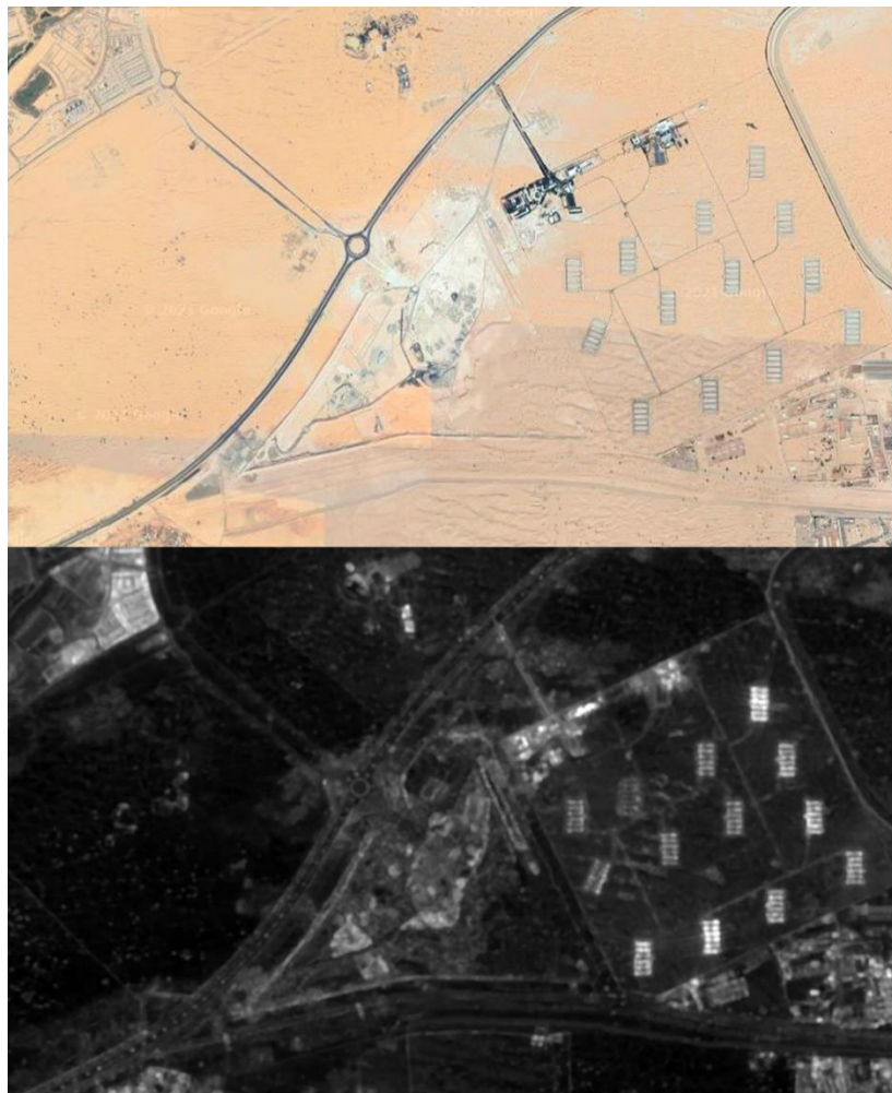
Figure 11.5 : The image is displayed in ground range and any measurement done on image are true to the ground
