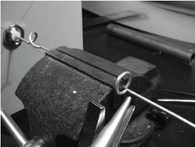
Figure AC 16: Repeat the stretching procedure for all of the remaining coils.
