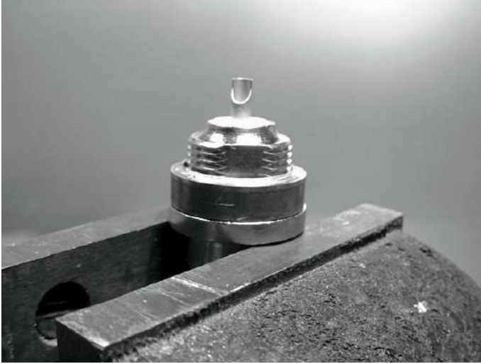
Figure AC 11: Adding a copper pipe spacer helps to match the impedance of the antenna to 50 Ohms.
