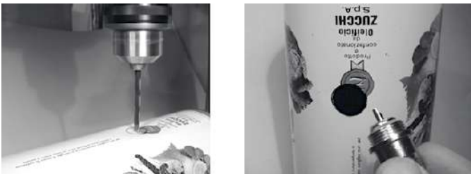
Figure AC 24: Carefully drill a pilot hole, then use a larger bit to finish the job.
