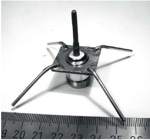
Figure ATL 11: Quarter wavelength ground plane antenna.
