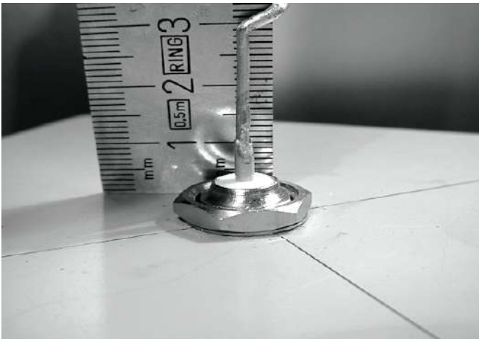
Figure AC 14: The first coil should start 3.0 cm from the surface of the plate.
