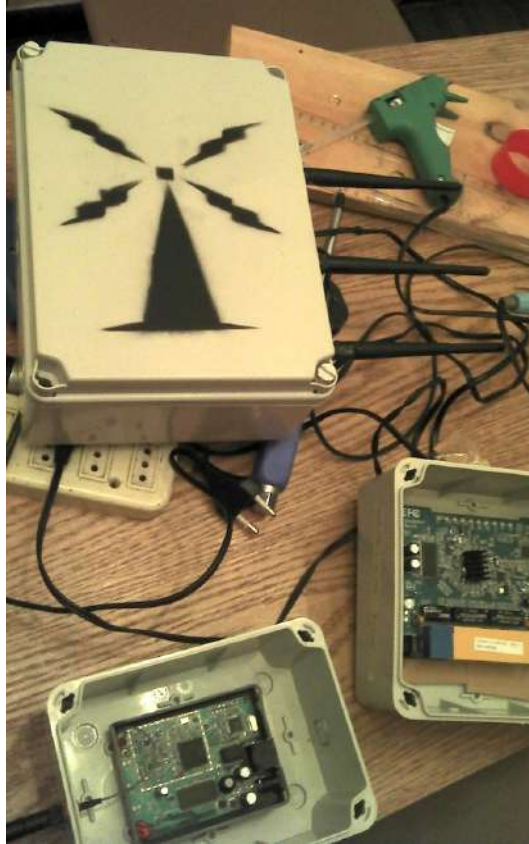
Figure MN 4:DIY outdoor routers based on PCBs taken from SOHO routers (Picture showing two devices based on TP-Link WR741 and WR941 and one based on a Fonea router)
