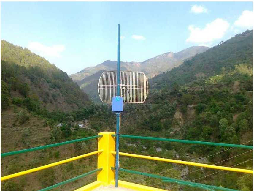
Figure CSD 10: Client Relay, Kangra Valley Network
