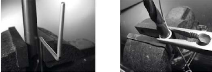
Figure AC 5: Bend the wire around the drill bit to make a coil.
